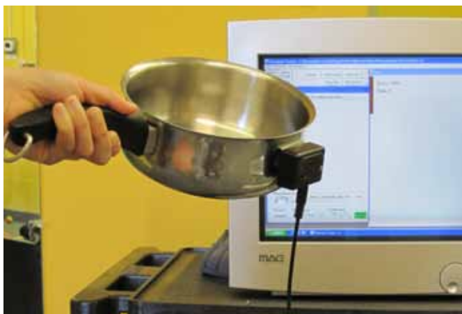
Figure 2: A tilt sensor attached to the saucepan detects movement.
