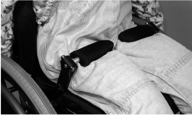
Figure 1 EPP positioned over child's upper thighs, below anterior superior iliac spines to provide secure pelvic stabilization in seating.
