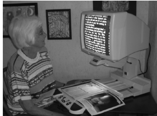
Reading magazines, financial documents or microwave food packaging can become possible again with a closed circuit television shown here in reverse polarity to provide white text on black background.
